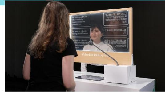
Examples of UC technology (Speech is translated or converted to text and displayed on a transparent display in real time)
